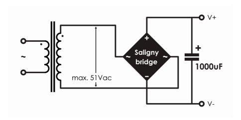
Variant b) - Full wave dual identical secondaries in parallel.
