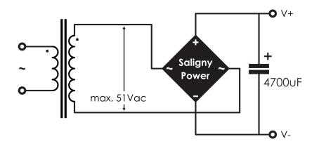
Variant B - full wave dual identical secondaries in parallel.
