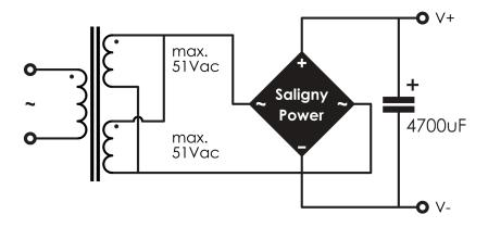
Variant C - Full wave rectification, for differential power supply, with two secondaries.
